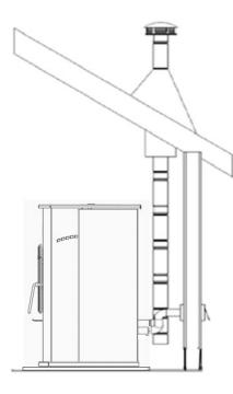
• Venting through the ceiling/roof may be the only feasible venting option in some cases and is a factory recommended installation.
