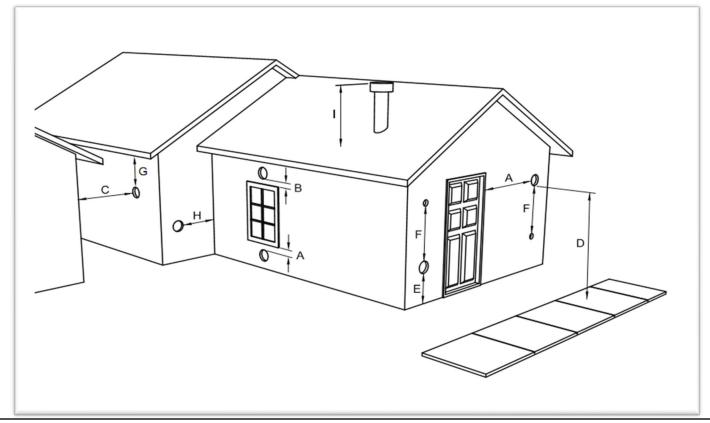
Notes on termination of Pellet Vent Pipe from NFPA 211 (2006 ed.) Section 10.4 Termination: 10.4.5 (See also "INSTALLATION" section of manual AND additional notes above):
