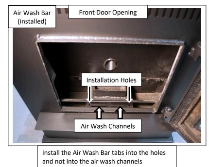
The Air Wash Bar should fit into the two installation holes and 'lean forward' on the front wall of the stove.
