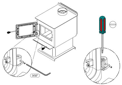
Using a flat screwdriver, turn the adjustable hinge rods in the direction shown to adjust the doors. Tighten all door hinge pressure screws when they are at the desired positions. Configurations 1-2-3-4-5-6, show in which direction these act on the adjustment of the door.
