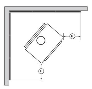
Figure 14: Heat shield clearances
