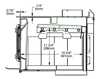
Figure 6: Side View - Combustion Chamber
