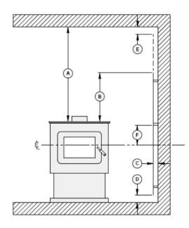
Figure 11: Heat shield clearances
