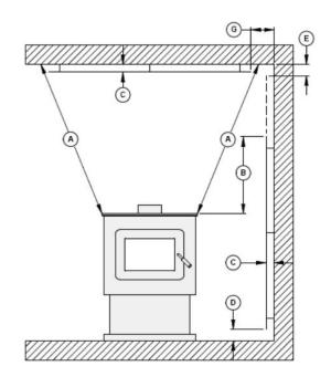
Figure 12: Heat shield clearances
